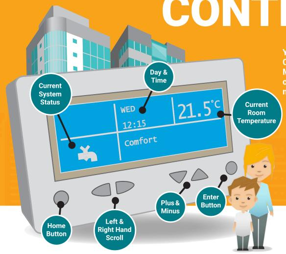
Your home features a ViewSmart Room Controller, which communicates with your ModuSat® heat interface unit, and allows you to control your heating & hot water and view your meter readings.
