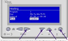
4. Here you can create a schedule. Use the Right Hand Scroll Button to highlight the values and the + & - Buttons to scroll through the Days, Times and Modes. (The example above shows a schedule for the Heating to operate in Comfort Mode Mon - Fri between 7am-9am)
