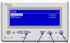
4. Here you can change the Mode for the Heating or Hot Water by using the Right Hand Scroll and then the + and - buttons to scroll through to the desired mode. (Note: when Comfort mode is selected the system runs 24/7 as per the setpoints).
