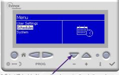
2. Select "Schedules" by scrolling down using the – button and pressing the Right Hand Scroll button to enter the menu.
