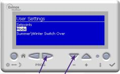
3. Select "Mode" by scrolling down using the – button and press the Right Hand Scroll button to enter the Mode menu.
