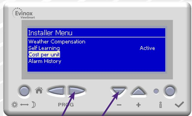
2. Select "Cost per unit" by scrolling down using the - button and pressing the Right Hand Scroll button to enter the menu.
