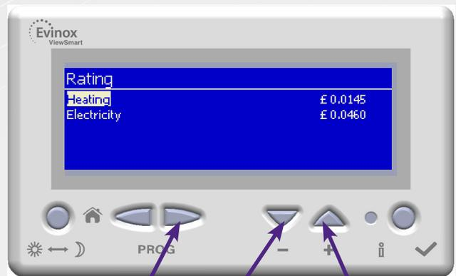
3. From here you can set the tariff rate. Scroll down using the - button and press the Right Hand Scroll button to select the type of meter (i.e Heating, Electricity)
