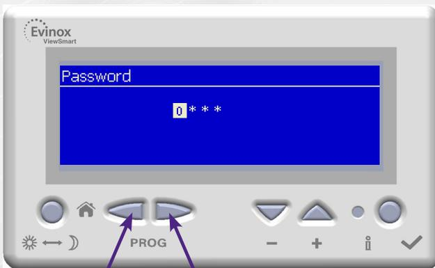
1. From the Home Screen - Hold down the Left & Right Hand Scroll buttons together for 3 seconds.
