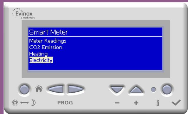
1. From the Main Menu Scroll down using the - button and select "Smart Meter" using the Right Hand Scroll button.
